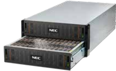
NEC SSE584 - 5K SAS enclosure with 84 x 3.5" drives
